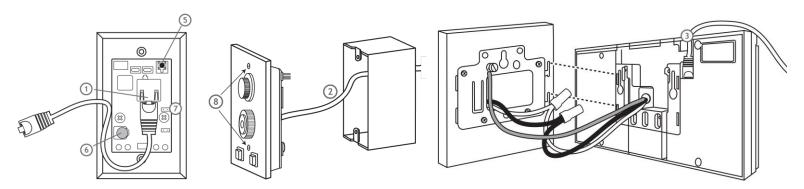
\*Use RJ45 Y-Splitter (part no 41270) to daisy chain more than one digital timer.
